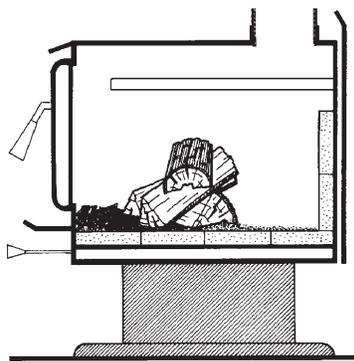
Figure 7: A small, criss-crossed load for mild weather
