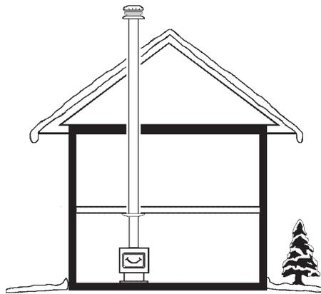
*Figure 1: This chimney and flue pipe arrangement gives the best performance*
