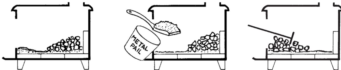
Figure 6: Left, coals at back, ash at front; centre, removing ash; right, raking coals
