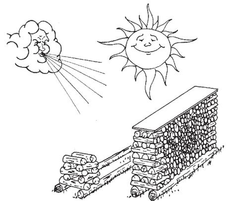
Figure 4: Stack wood on rails in an open area
